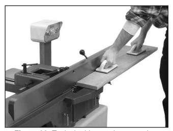
Figure 28. Typical rabbet cutting operation.
